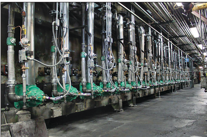
Furnace after conversion with Eclipse 8" SER v5 burners.
