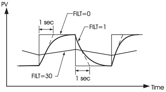
Figure 3.8 Filter Characteristics
