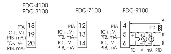
Figure 2.8 Sensor Input Wiring
