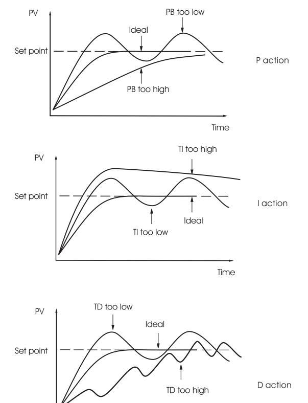
Figure 3.9 Effects of PID Adjustment
