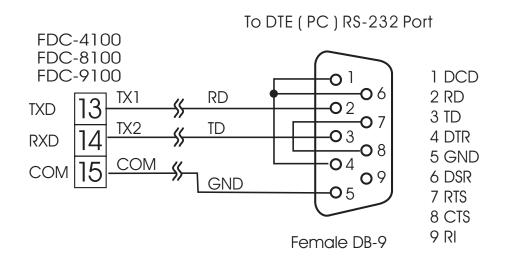
Figure 2.21 Configuration of RS-232
