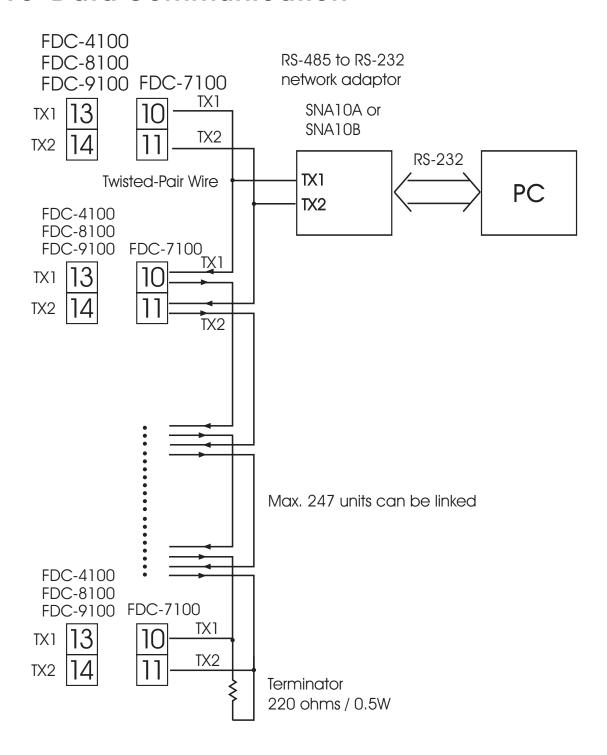
Figure 2.19 RS-485 Wiring
