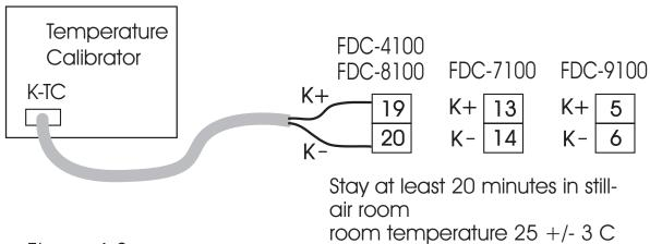
Figure 4.2 Cold Junction Calibration Setup
