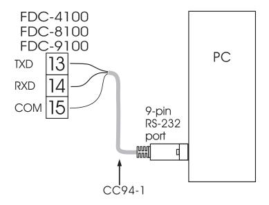
Figure 2.20 RS-232 Wiring
