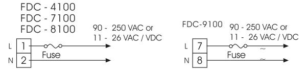
Figure 2.7 Power Supply Connections
