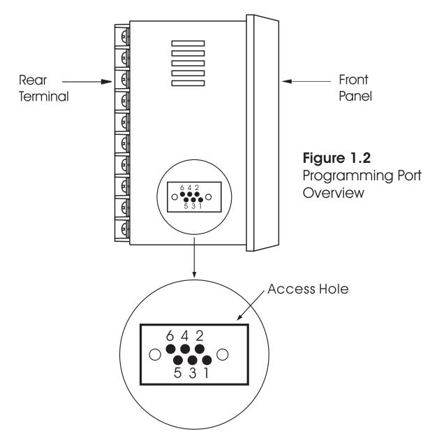
A special connector can be used to touch the programming port which is connected to a PC for automatic configuration, also can be connected to an ATE system for automatic calibration and testing.
